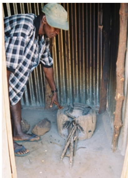
Fuel-efficient wood stove produced by Environmental Foundation for Africa (EFA) in Sierra Leone.
