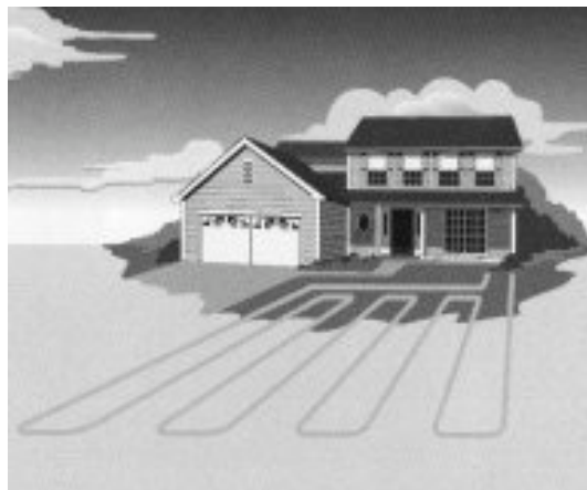
Example of horizontal loop system.
